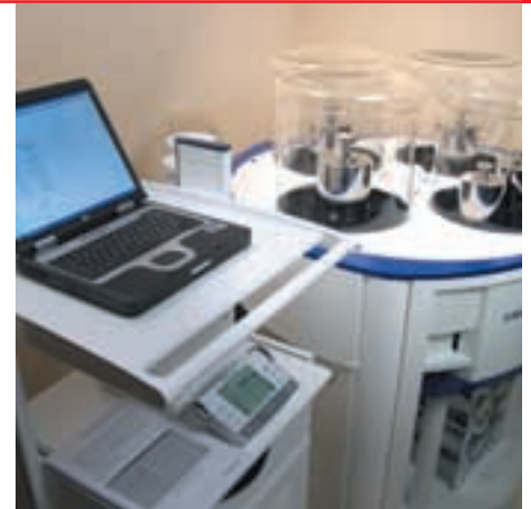
Troemner's New Mettler Toledo, Inc. AX64004 Mass Comparator for 10 kg—60 kg Weights
